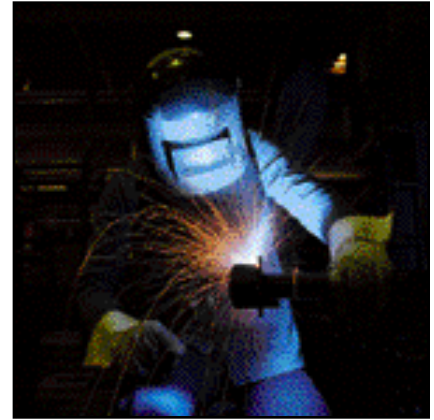
GTAW and GMAW welding processes are utilized on nozzles and end frame reinforcing bars, respectively.
