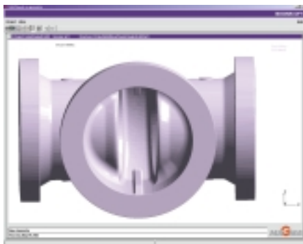
Pro-Engineering model imported into Magmasoft® casting simulation program.
