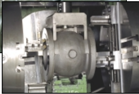
For smaller runs, complete automatic machining and drilling in one set-up.
