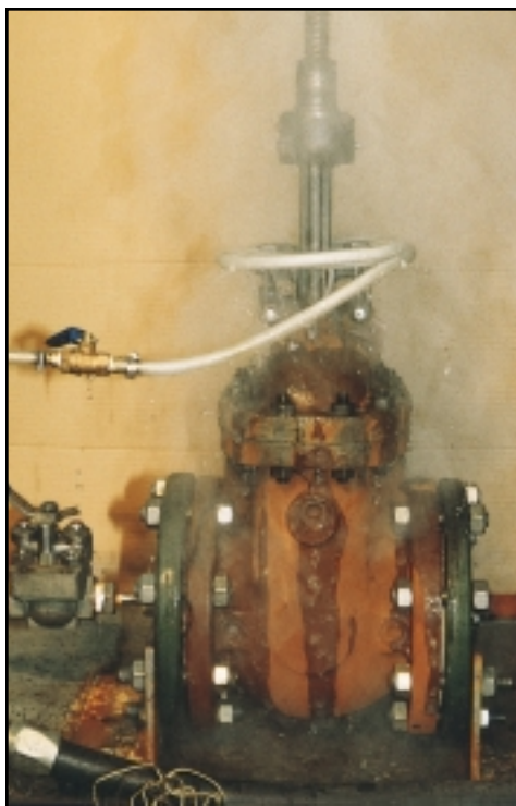
Upper left: 3000 cycles with propane at 125 psi Leakage: zero ppm.
