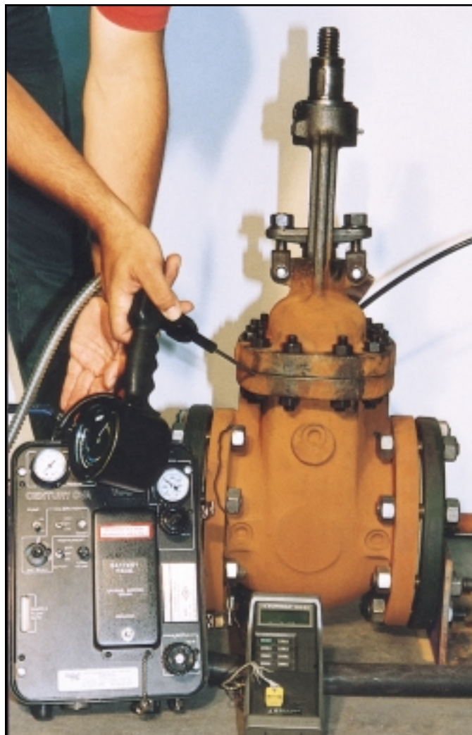
Upper right: 50 cycles with steam at 400°F (204°C) Leakage: zero ppm.
