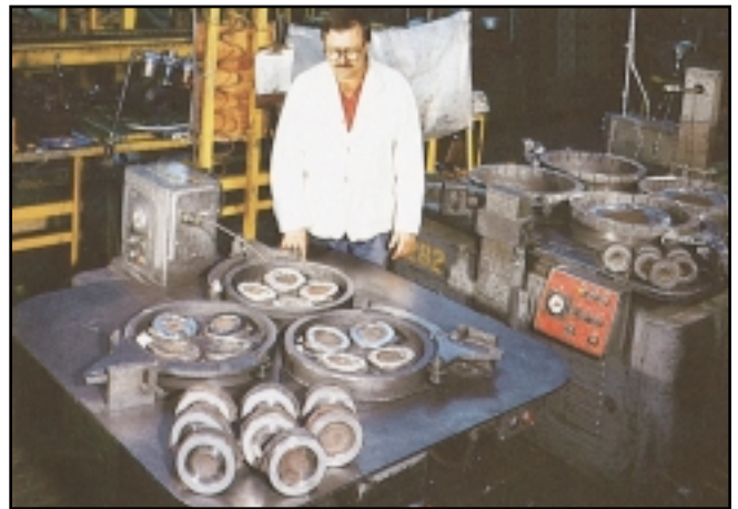
6 Lapping of wedge seating surfaces.
