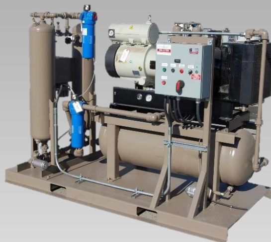
Instrument air compressor package using a 30HP Mattei rotary vane compressor with wet air receiver, filtration, twin-tower heatless regenerative air dryer and compressor control panel.
